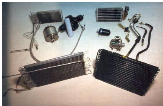
R744 lab. prototype system (left) and BMW 520 CFC-12 system (right)
